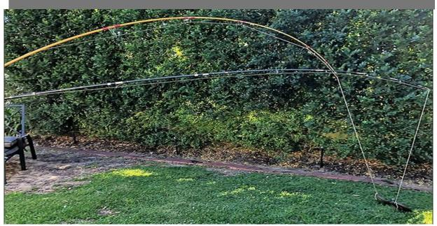
**Caption**: The difference in pulling power graphically demonstrated with a mere 2.5kg hanging off the rod tip. Old school fibreglass versus powerful graphite.
