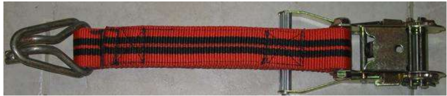
Ratchet end of a typical strap set.
